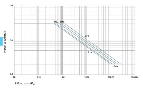
As a result, if cushionings can not absorb the kinetic energy and changing the working parameters is not possible, it is necessary to provide an additional hydraulic shock absorber (YDA / YDR series) to reduce the load speed before the cushionings operate.
