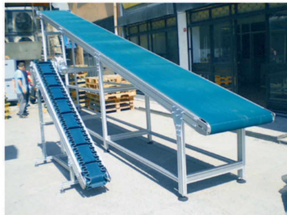
Graded Conveyor and Elevator
